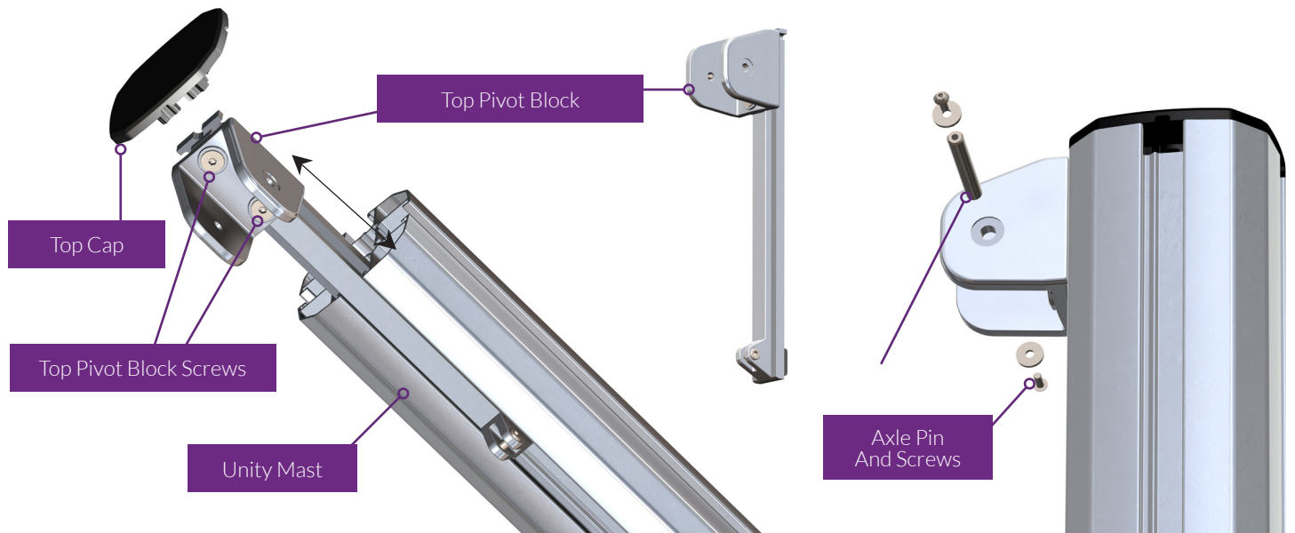
Figure P - Mounting Additional Frames(s)
